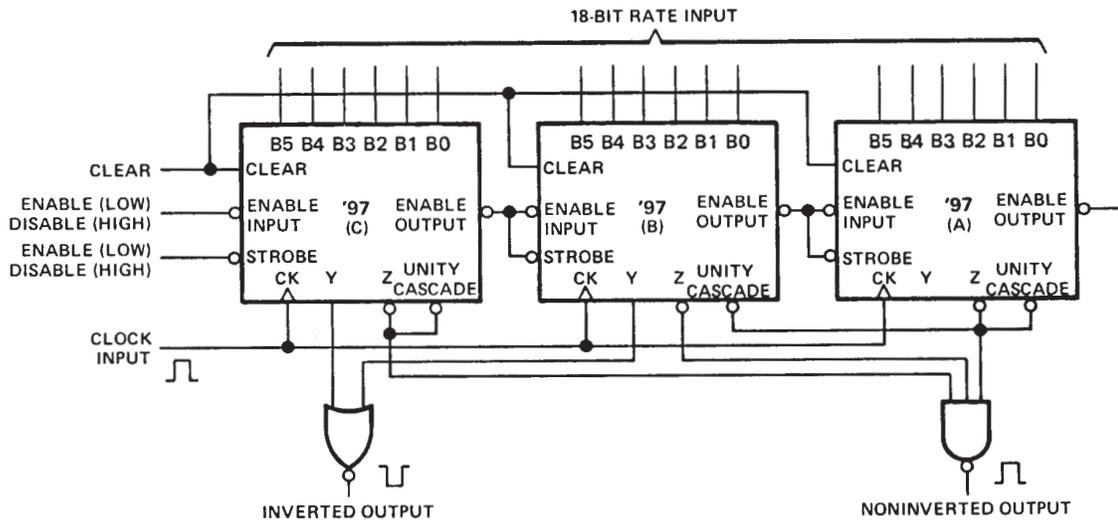
As illustrated, two of the 6-bit multipliers can be cascaded by connecting the Z output of unit A to the unity cascade input of unit B, in which case, a two-input NOR gate is used to cascade the remaining multipliers. Alternatively, all three Y outputs can be cascaded with a 3-input NOR gate. The three unused unity cascade inputs can be conveniently terminated by connecting each to its Z output.
