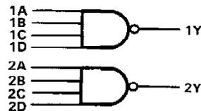
positive logic  $Y = \overline{A \cdot B \cdot C \cdot D}$  or  $Y = \overline{A} + \overline{B} + \overline{C} + \overline{D}$
