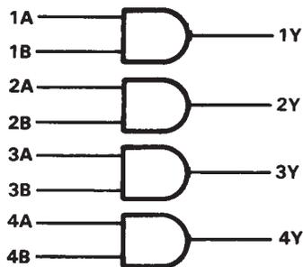
$$Y = A \cdot B \text{ or } Y = \overline{\overline{A} + \overline{B}}$$
