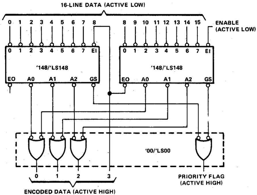
Since the '147/'LS147 and '148/'LS148 are combinational logic circuits, wrong addresses can appear during input transients. Moreover, for the '148/'LS148 a change from high to low at input EI can cause a transient low on the GS output when all inputs are high. This must be considered when strobing the outputs.
